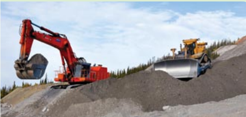
The darling of the construction project is the Caterpillar's D11R dozer, the largest machine on-site. This machine is so big that it was disassembled and transported to the Yukon on three tractor trailers. Photo: Government of Yukon
